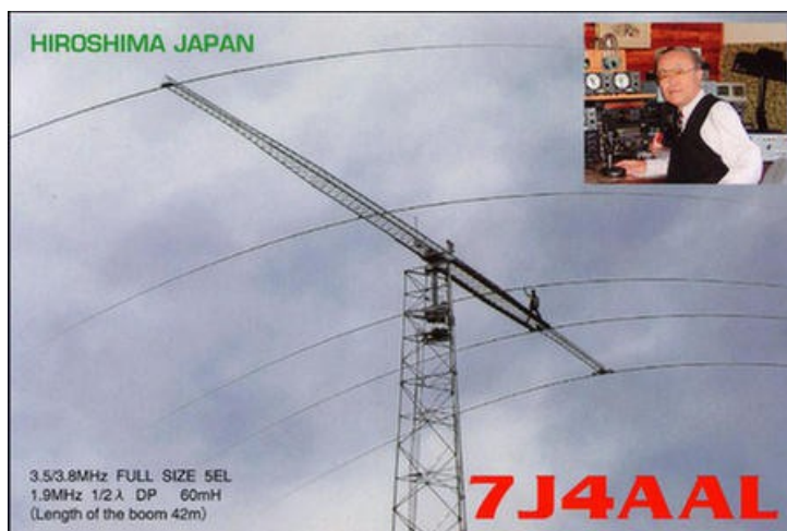
That's a man standing on the boom, near the driven element
