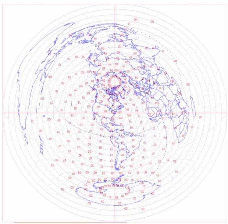
By plotting the signal paths from our location as straight lines, like spokes on a bicycle wheel, we get this chart. Here, distances from our location and directions along the Earth's surface are shown in correct proportion and direction, but only from our perspective. Note that the direction of a signal from here to Japan is now shown correctly as NNW, but Australia is now so badly distorted it's hard to recognise. It's that huge shape in the upper left.
