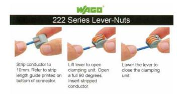
I recently learned of a new electrical product for splicing wiring. It is called Wago 222 Series Lever-Nuts. They are rated for at least 20 amps and accept wire sizes of AWG 28 to AWG 12. I use them for joining
