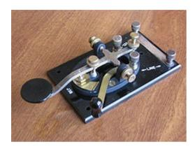
A typical "straight key." This U.S. model, known as the J-38, was manufactured in huge quantities during World War II, and remains in widespread use today. In a straight key, the signal is "on" when the knob is pressed, and "off" when it is released. Length and timing of the dots and dashes are entirely controlled by the operator.
